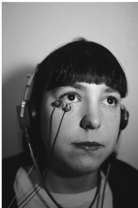
Figure 9.6 Apparatus used to measure eye-blink startle reflex in human beings. Two recording electrodes are placed on the orbicularis oculi (eye-blink) muscle (a third is placed either on the forehead or on the bone behind the ear, the mastoid, to form a ground). Acoustic startle stimuli are presented over headphones.
